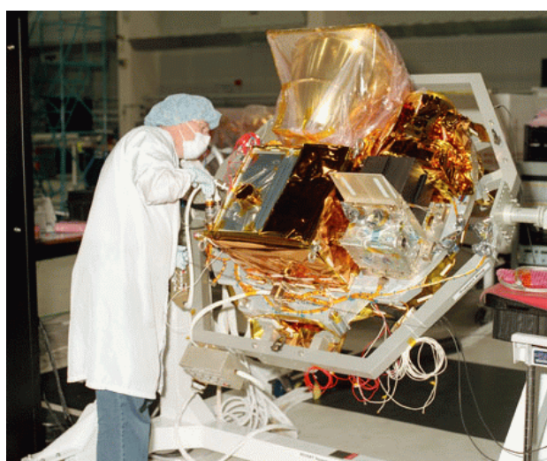
Figure 14: SciSat undergoing final assembly at the David Florida Laboratories in Ottawa. The satellite was subsequently shipped to Vandenberg AFB to be launched on a Pegasus launch vehicle.
