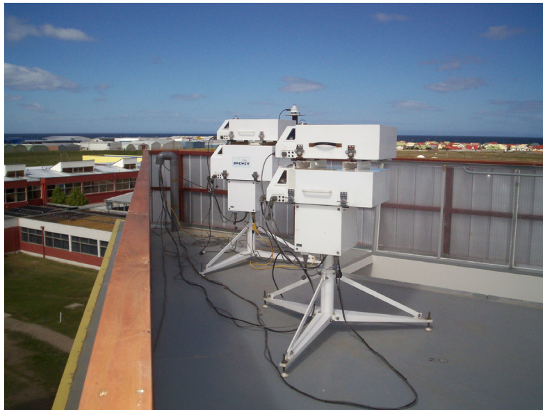
Figure 1: Brewer MKIII #180, MKIV#124, MKIV#068 and the traveling Brewer MKIV#017, during the calibration activities at Punta Arenas.
