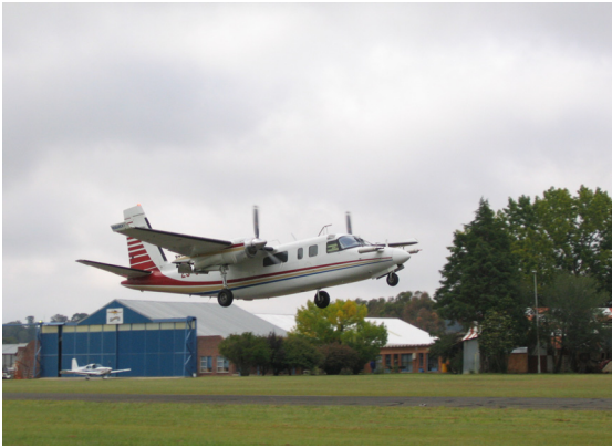
Figure 3: SAWS research Aircraft and under-wing measurement pods.
