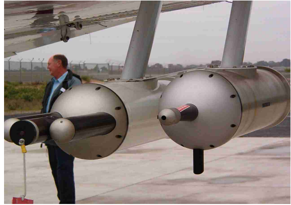
Figure 3: SAWS research Aircraft and under-wing measurement pods.
