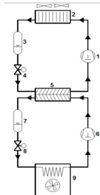
1: high temperature compressor, 6: low temperature compressor, 2: air condenser, 3 and 7: refrigerant receivers, 4 and 8: Expansion valves, 9: low temperature evaporator, 5: evaporator-condenser
