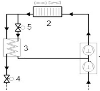
1: compressor, 2: air condenser, 3: economizer, 4 and 5: Expansion valves
