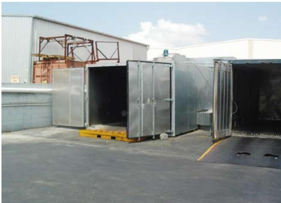
*Modified containers (Kilquick, Brisbane) used for heat treatment to ISPM No. 15 (J. Banks)*
