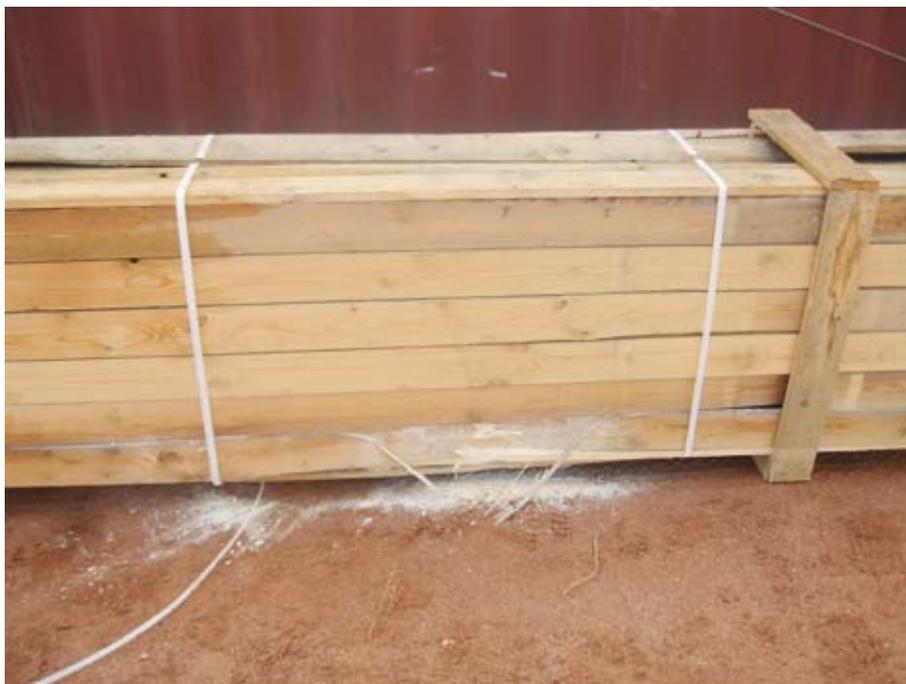
*Damage to timber packaging material, showing presence of quarantine pests at import. Treatment with methyl bromide or alternatives required (AQIS, Australia)*
