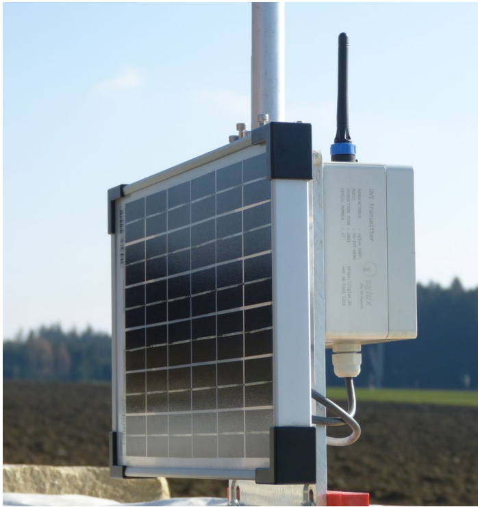
Figure 6. Self-contained broadband radiometer with solar panel Credit: Markus Laufmann; © Federal Office for Radiation Protection (BfS)
