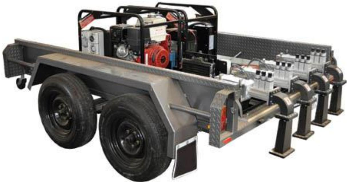
**Figure 1.** Prototype unit under evaluation to disinfestation soil using microwave at Toolangi, Victoria.
