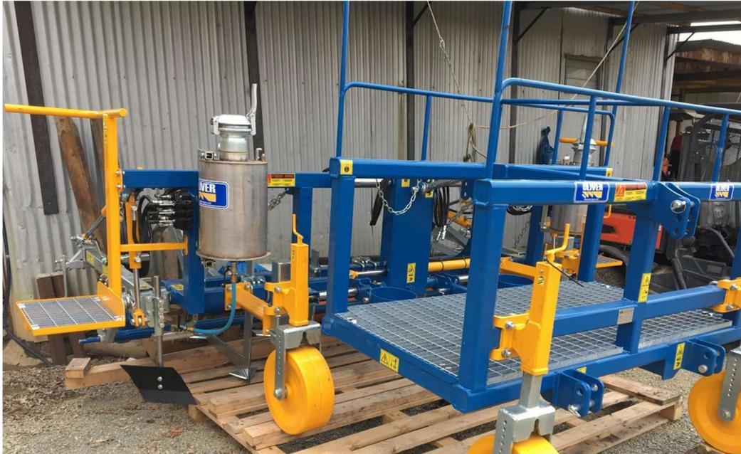
**Figure 1.** New rig for applying fumigants in the strawberry runner industry. The design incorporates swept back tynes and small duck-feet for minimising the losses of volatile fumigants like EDN from soil, longer tynes for injecting fumigants at greater soil depths, and a hot-glue system for welding sheets of totally impermeable film.
