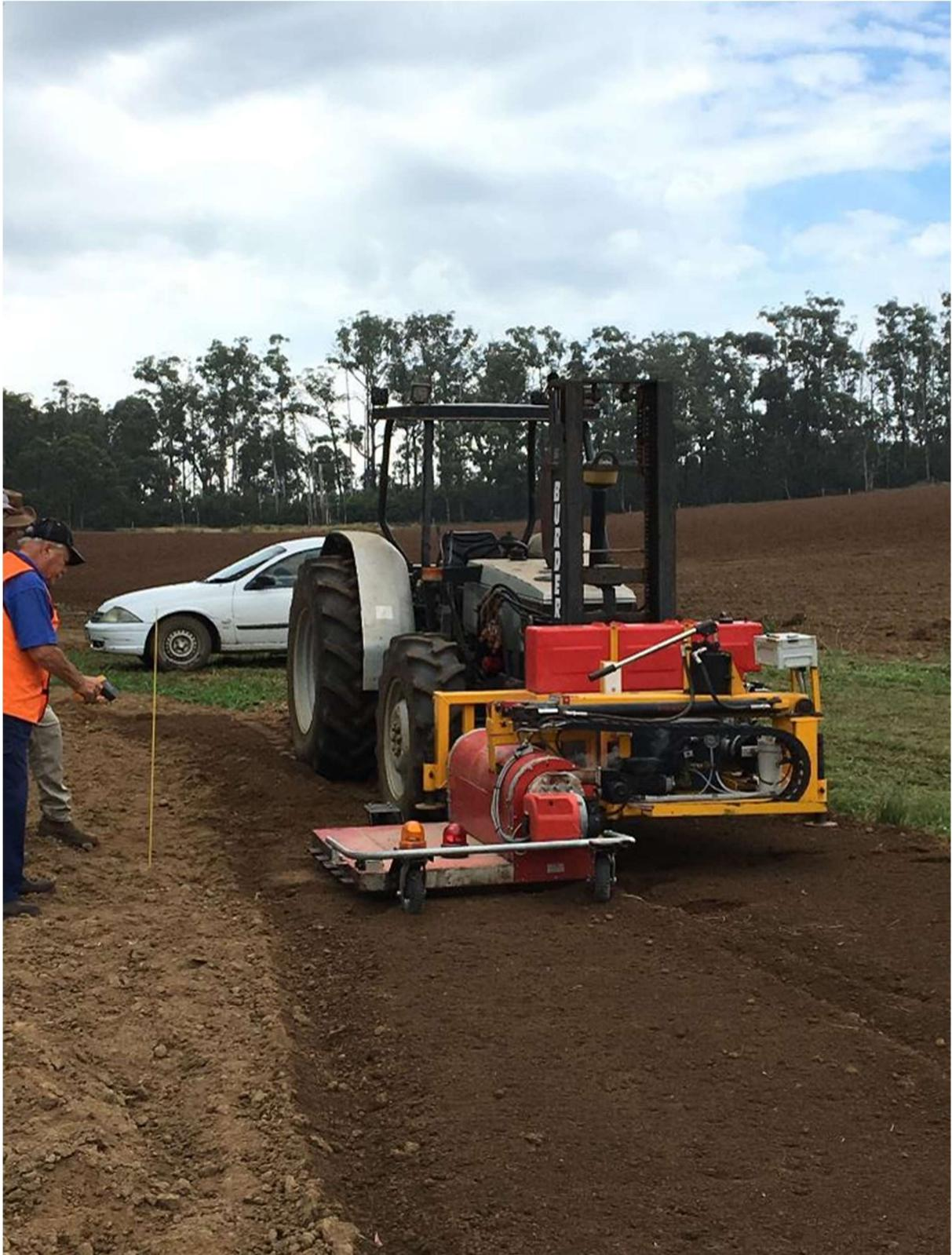
**Figure 3.** Small-scale steam rig used to treat soils at Toolangi in trials conducted in 2017/18.
