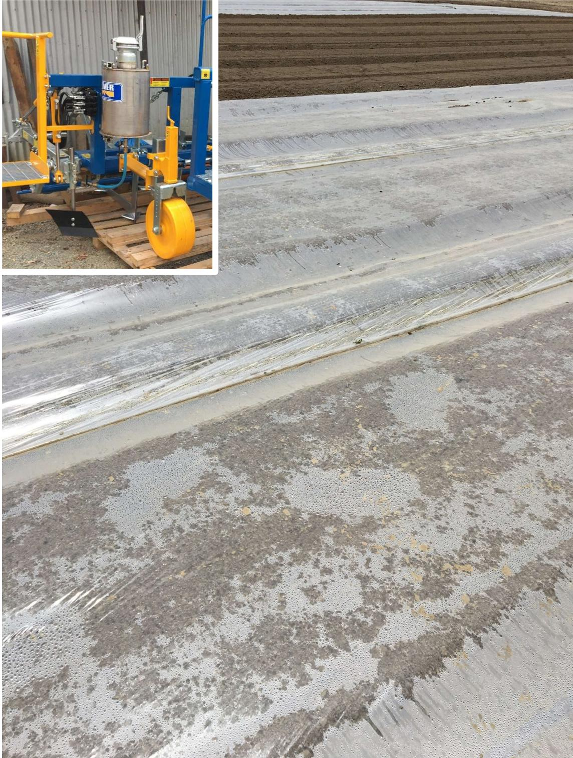
**Figure 1.** New trial evaluating hot-melt systems for joining TIF plastic for broad-acre application of substitute fumigants and lower rate MB/Pic (Draslovka Services Pty Ltd).
