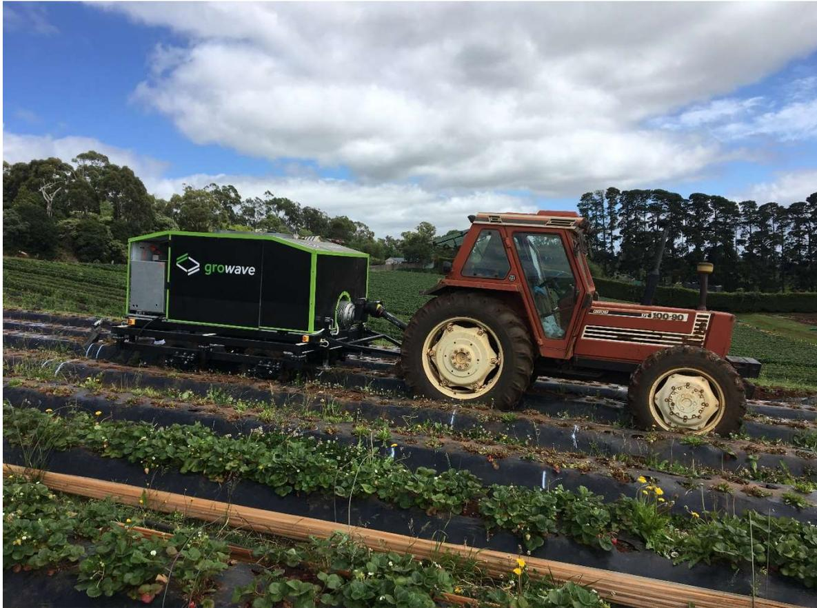
**Figure 2.** New microwave rig with greater power (5 kW) that is being evaluated for soil disinfestation in the strawberry runner and fruit (above) sectors (GroWave Pty Ltd).
