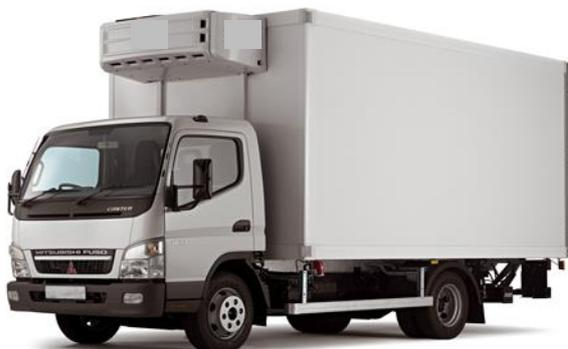
*Small refrigerated truck, compressor located by main vehicle engine*
