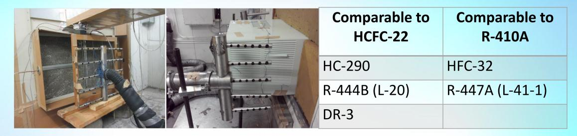
13 custom-built prototypes in four categories ranging from 5 to 27 kW, testing five different alternatives against the baseline refrigerants HCFC-22 and R-410A
