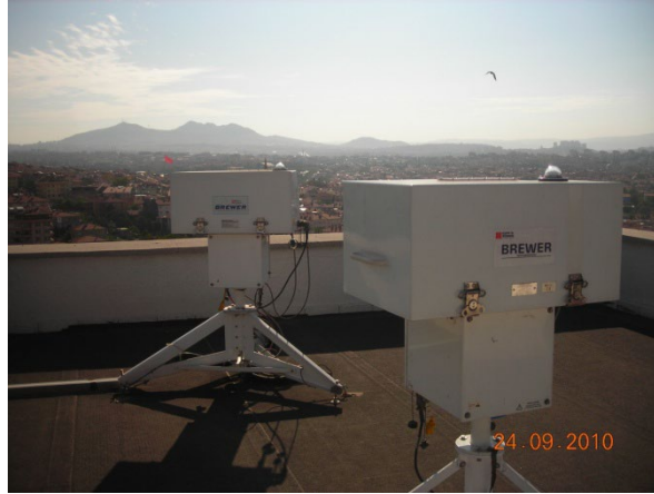
Figure 3. Second calibration of Brewer MKIII #188 with the reference Brewer MKIII #158 in Ankara station.
