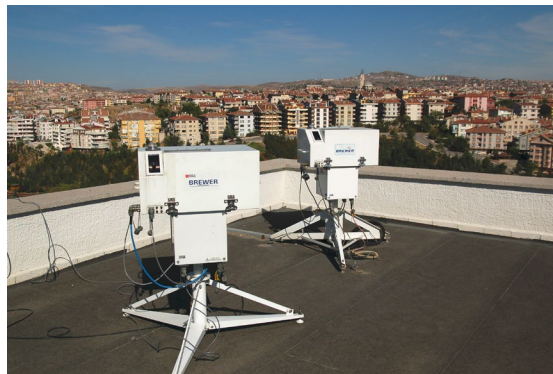
Figure 4. Third calibration of Brewer MKIII #188 with the reference Brewer MKIII #158 in Ankara station.
