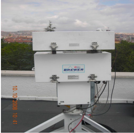
Figure 2. First calibration of Brewer MKIII #188 with the reference Brewer MKIV #017 in Ankara station.
