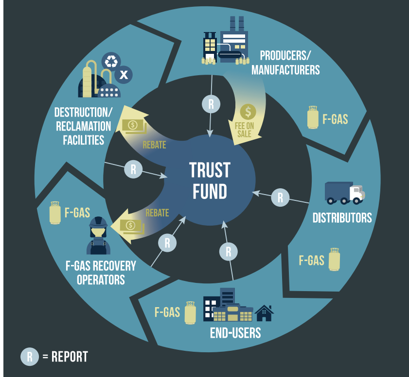
Figure 4: Under an extended producer responsibility scheme a fee on the sale of F-gas or F-gas products finances a rebate for recovery, collection, transport and reclamation/ destruction.
